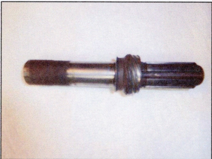
The speedo gear frozen solid to the drive shaft
