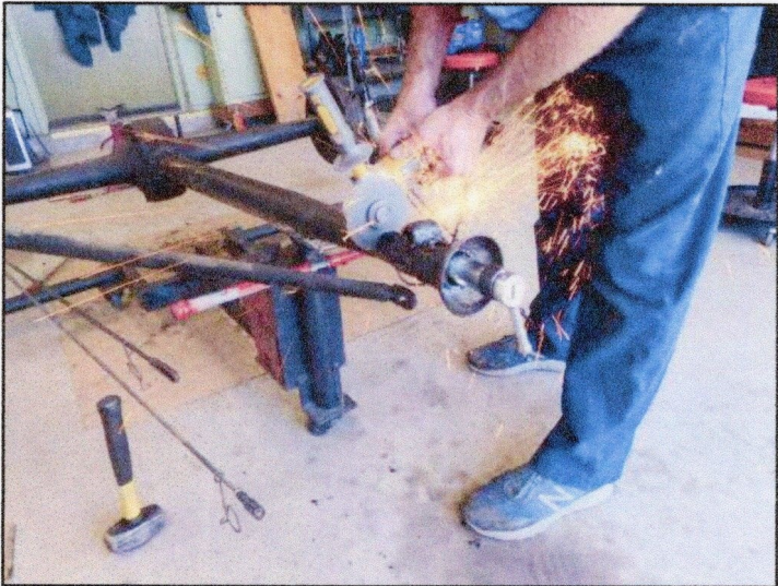
The front of the torque tube was sawed off
