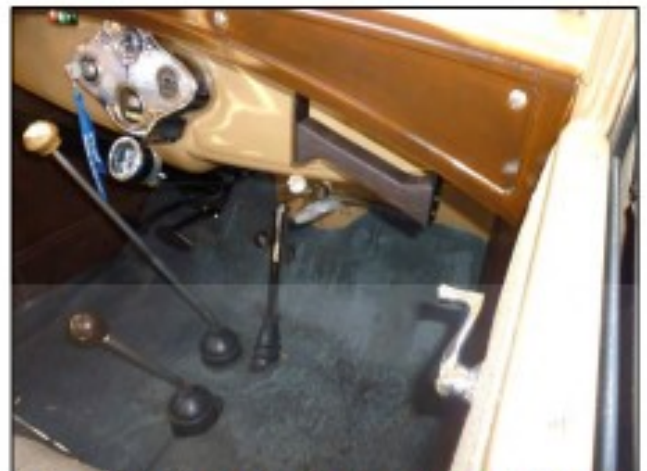
The grabber is attached using existing bolt holes
