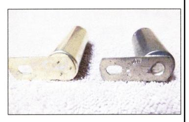
On the left is a good quality Bratton's condenser. On the right is a poor quality soldered on condenser still being sold by some suppliers.
