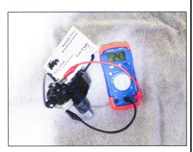
The Honeytek tester is a unique thing to have along on a tour. You can easily test a condenser while it is still attached to a distributor installed in a Model A. Simply remove the car's fuse, and slip a business card between the points. The plus lead of the tester is clipped to the arm of the points; the negative lead is clipped to ground on the distributor.
