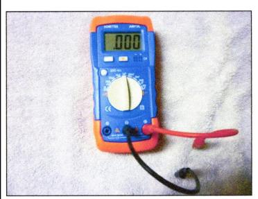
A Honeytek A6013L Capacitor Tester (called a condenser in automotive jargon) is available through Amazon for about \$22. The tester will tell you not only if the condenser is good or bad, but the actual value in micro-farads. Set the pointer on two micro farads.
