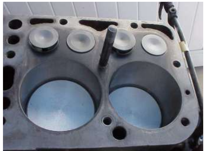
The area between #3 and #4 cylinder is a common place for a blown head gasket. The #8 stud sits right next to the area.
