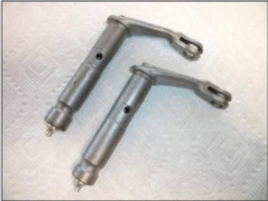
The above photo shows a grease fitting in service on a vehicle driven daily. Give it a shot of grease whenever greasing the car.
