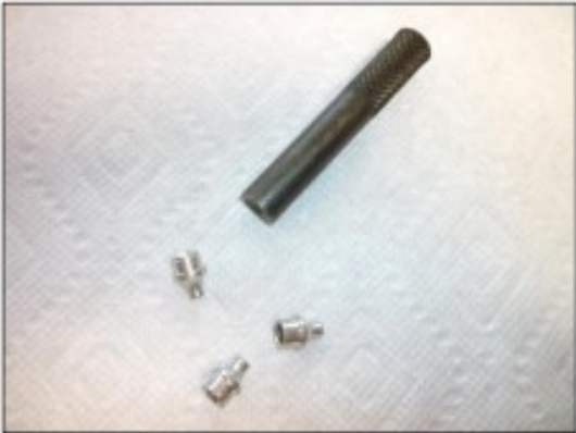
Press in type grease fittings and the insertion tool
