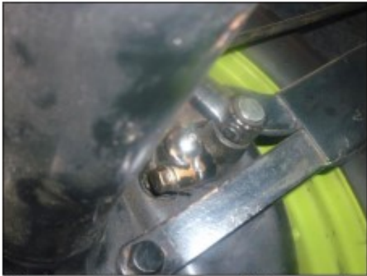
The above photo shows a grease fitting in service on a vehicle driven daily. Give it a shot of grease whenever greasing the car.
